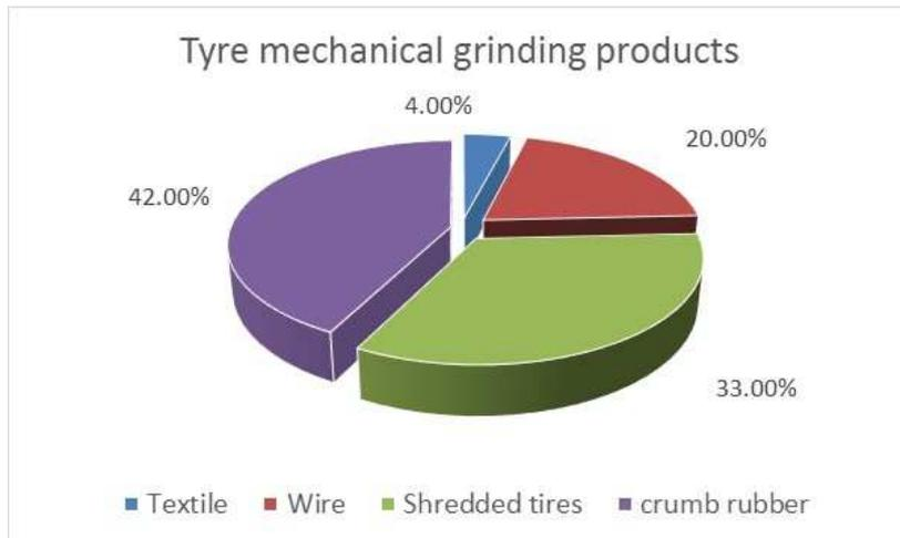
Fig.2. Products from mechanical grinding process.
