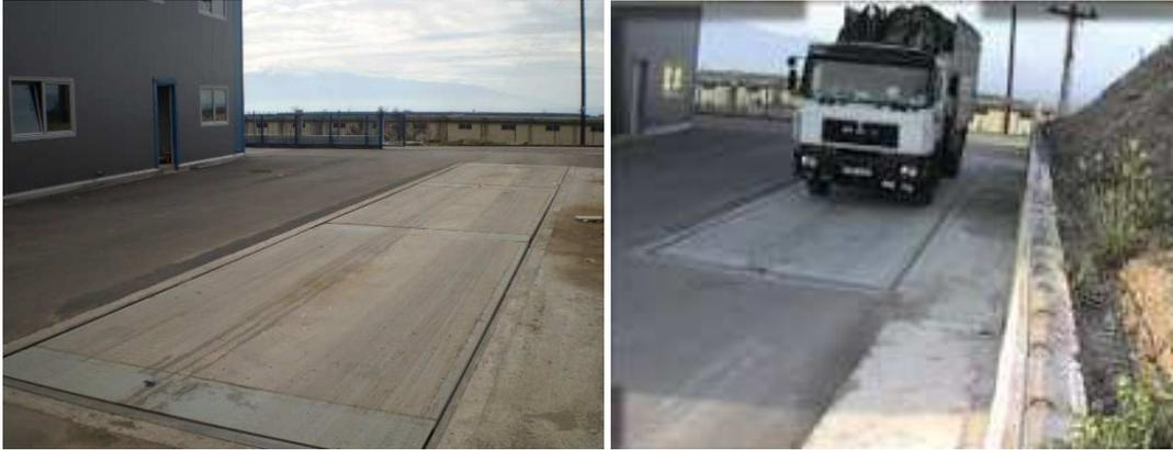
Fig.3. Weight bridge installed in plant in order to collect and transmit online data
